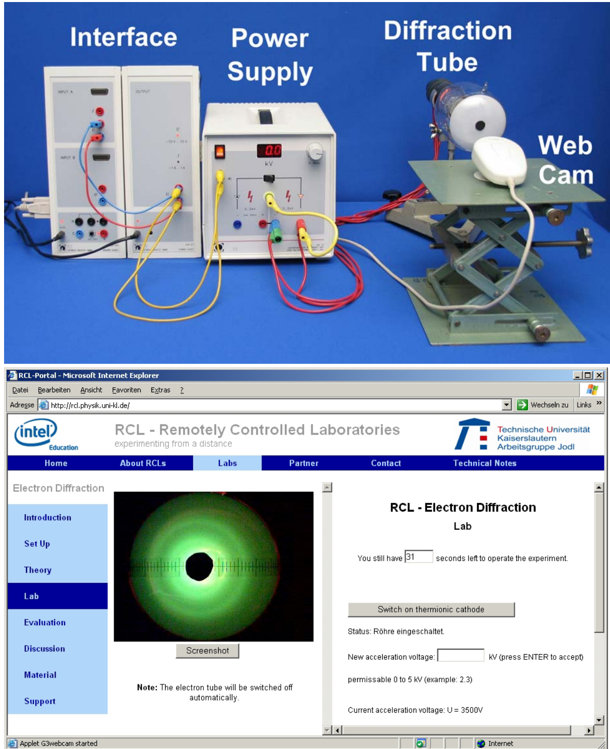
Fig. 2: RCL „Electron Diffraction“: experimental set up with CASSY-interface [18, 19], power supply, electron tube and web cam (top). Screenshot of the website under menu option „Lab“: live video stream (the diffraction order 0 is blocked to avoid supersaturation of web cam) as well as chosen acceleration voltage and some other data (bottom).
