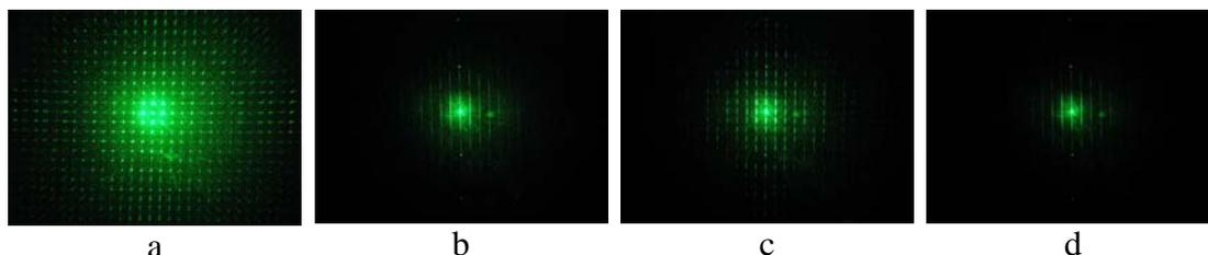
**Fig 2.** Diffraction pattern of 2x1 (a), 50x1 (b), 50x2 (c) and 50x50 (d) holes in a rectangular square lattice, respectively.
