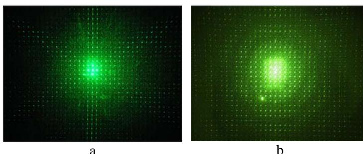
**Fig 3.** Diffraction pattern of a square lattice with circular holes (a) and hexagons (b).
