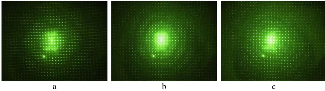
**Fig 4.** Diffraction pattern of a square lattice with increasing circle diameter from (a) to (c).
