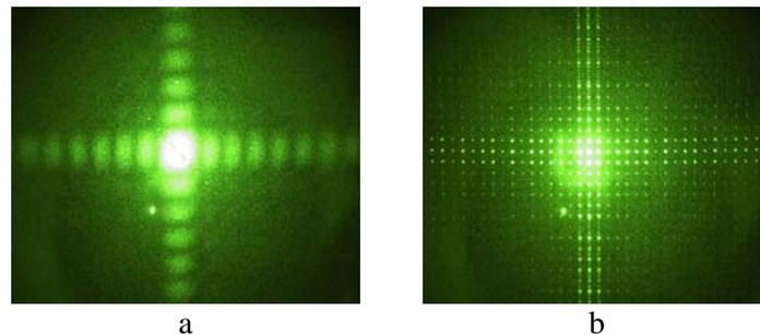
**Fig 5.** Diffraction pattern of a square lattice build by squares of zero variance (a) and statistical deviation from perfect lattice points (b).
