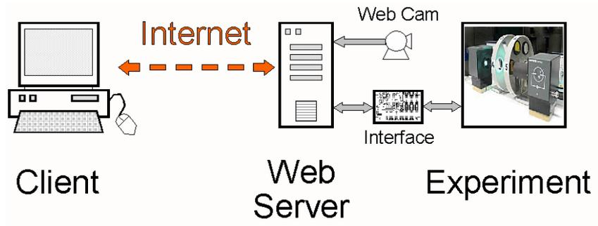
**Figure 6.** Simplified schematic sketch of a remote lab.
