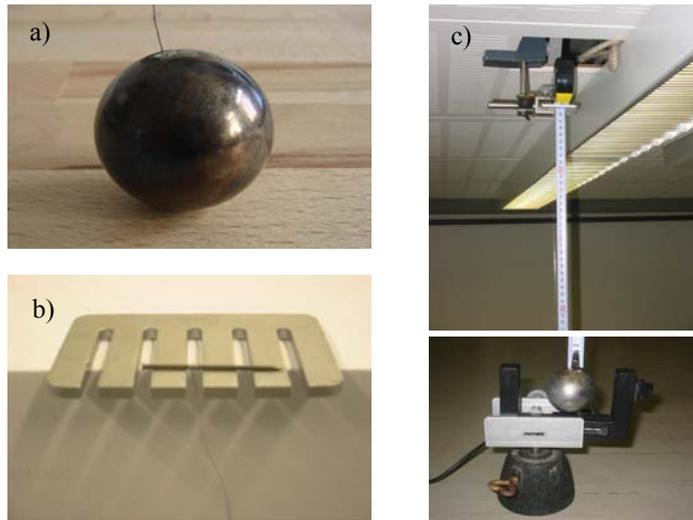
**Figure 4.** Sphere of the pendulum with soldered wire (a), suspension of the pendulum by means of a pin mounted on a comb (b), determination of wire length by a pocket tape measure (c).
